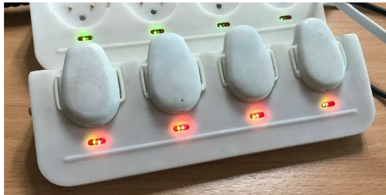
Figure 7. AiR node for monitoring activity and behavior parameters of patients.
