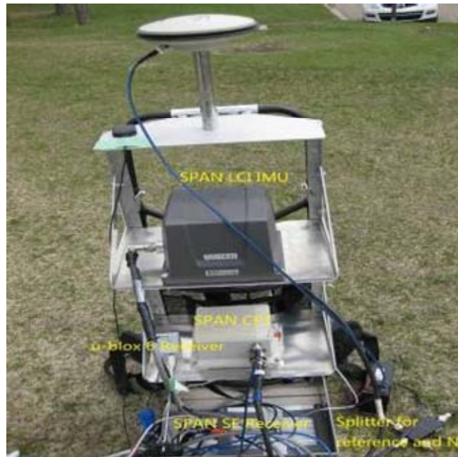
Figure 5.2: Data collection equipment in the backpack
