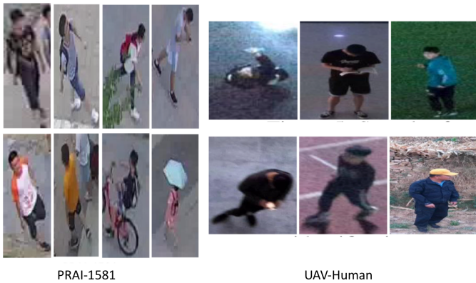
Figure 11: Challenges for aerial person re-ID due to elevation angle, blur, lighting/illumination, and occlusion. Images from two aerial person re-ID datasets: PRAI-1581 [177] and UAV-Human [80].
