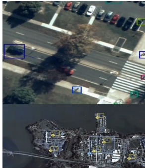
Figure 1: The rise of aerial surveillance. (1) The first column shows the military all-seeing Gorgon Stare [93] deployed in Iraq, using a MQ-9 drone (costs $17M USD) flying at an altitude of 25K feet, able to capture simultaneously an area of 10 \times 10 km, with a 1.8 GB sensor at a Ground Sampling Distance (GSD) of 15 cm. (2) The second column is Stratollite, a giant solar-powered balloon flying at an altitude of 65K feet [104], which can hover for months, able to detect a mobile phone in a person’s hand at a GSD of 5 cm. (3) The third column is the off-the-shelf DJI Mavic 2 (costs $3K USD) flying at an altitude of 1K feet, able to capture simultaneously an area of 1 \times 1 km, at a GSD of 20 cm [187].
