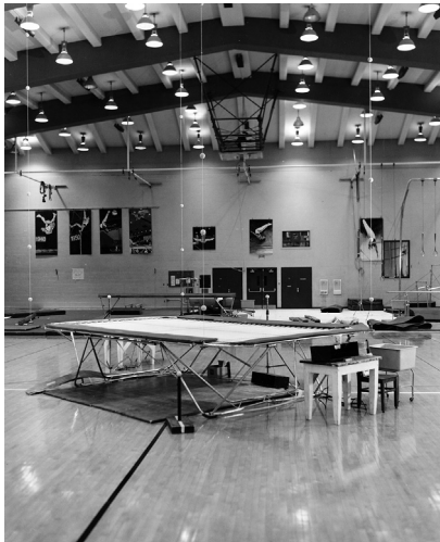
Figure 3 — Experimental set-up for motion capture at Penn State (1973). Note the Walton timer 1 on table in the foreground and the control points used for camera calibration.
