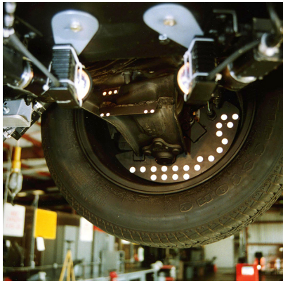
Figure 5 — Motion capture setup to measure the 3-dimensional kinematics of road wheels and steering linkage due to brake vibration (1997). The tests used 7 synchronized cameras to correlate steering wheel vibrations with the steering linkage and road wheel measurements. The tests were conducted on a 2-mile test track at speeds in excess of 100 miles per hour. Output also included dynamic camber, caster, and toe measurements.
