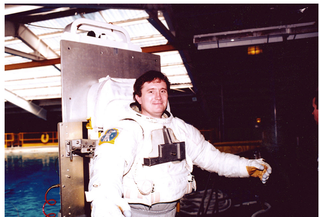
Figure 4 — Motion capture to determine the range of motion of space suits (1988). These tests were conducted underwater to simulate weightlessness, and (black) racquetballs were used to mark reference points on the space suits.
