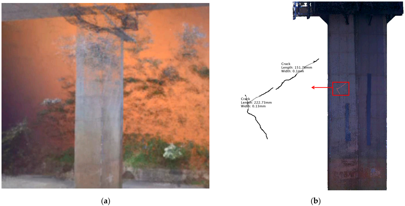
Figure 6. Scan-to-BIM model: (a) point cloud model generated using the photogrammetry algorithm using digital images acquired by a digital camera embedded on a UAV; (b) texture- and damage-mapped BIM model.
