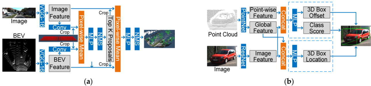
Figure 8. The representative detection methods using multi-stage feature-based fusion strategy. (a) AVOD; (b) PointFusion.
