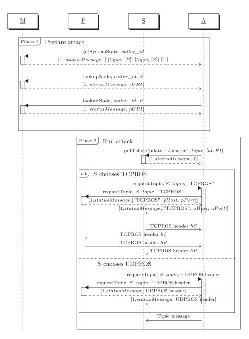
Figure 2.1: Sequence diagram of a stealth publisher attack
