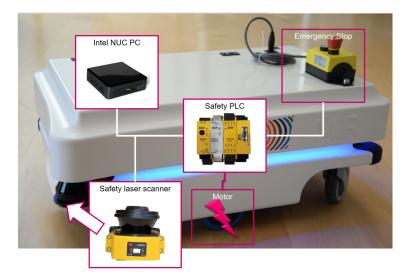
Figure 1.1: A logical overview of the internals of a MiR-100 robot (from [138])
