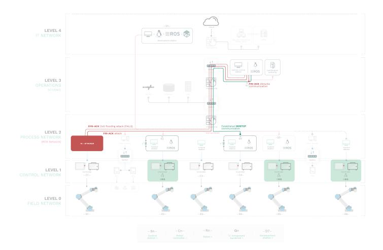
Figure 3.4: Architecture diagram depicting attacks to ROS via underlying network protocols. Depicts two offensive actions performed as part of  $A_2$ . The SYN-ACK DoS flooding does not affect  $\hat{S}_7$  due to hardening. In green, a previously established ROS-TCP communication between  $\hat{S}_4$  and  $\hat{S}_7$ . In red, the FIN-ACK attack which successfully disrupts the network interaction leveraging flaws in underlying network protocols.
