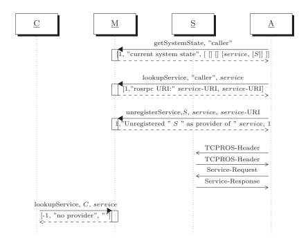
Figure 2.3: Sequence diagram of a service isolation attack
