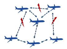
Figure 5.2: A team of UAV collaborate on a mission. They can communication with each other when one is in the range of communication of the other. An attacker can jam the signals between two UAV.
