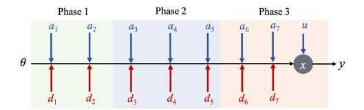
Figure 5.3: Multi-stage and multi-phase interactions between an attacker and a defender: The attacker changes the cyber state  $\theta$  to affect the physical state x at the last stage of Phase 3.
