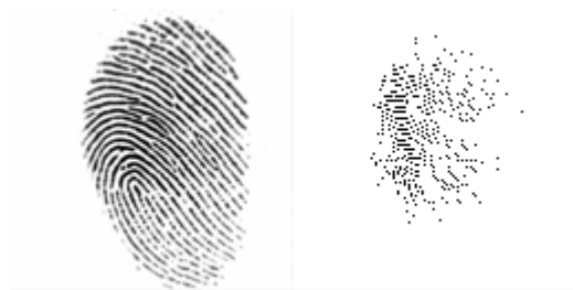
Figure 3.21: Original image and Roberts edge detection image (speed = 0.007443 seconds)
