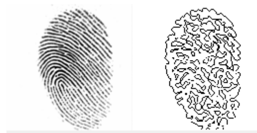
Figure 3.20: Original image and Laplacian edge detection image (speed = 0.018300 seconds)
