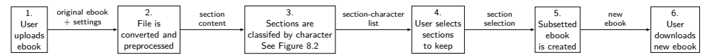
Figure 8.1: The full NovelPerspective pipeline. Note that step 5 uses the original ebook to subset.
