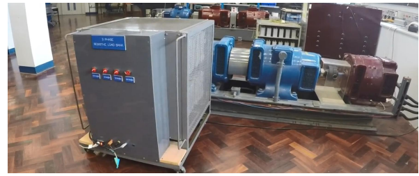
(a) Microgrid and 3-Phase Transmission Load
