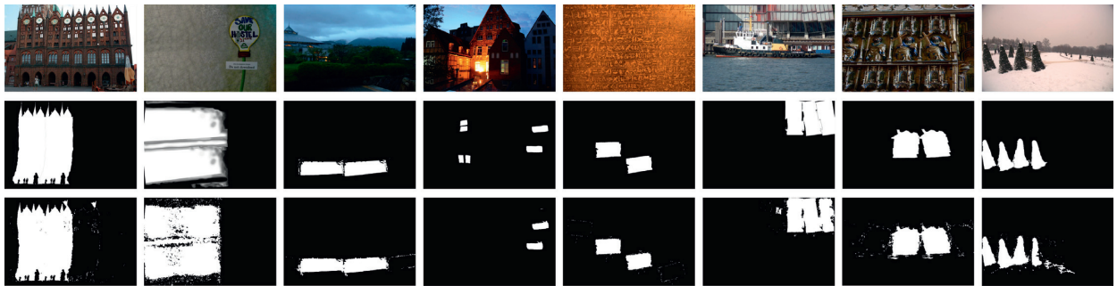
FIGURE 10: Copy-move forgery detection results for the rotation. Top to bottom: test images from dataset, ground-truth forged regions, and forged regions detected by the proposed algorithm. Left to right, the angle of rotation is 2°, 4°, 4°, 6°, 6°, 8°, 8°, and 10°.
