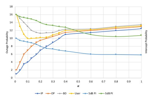
Fig. 3. Intercept and outage probabilities for various  $\alpha$  values
