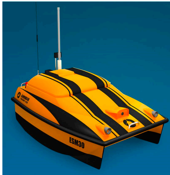
Figure 8. ESM30 autonomous water sampling and monitoring boat (Source: YUNZHOU TECH).
