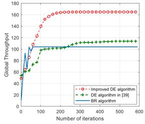
**FIGURE 10.** Global throughput vs. the number of iterations in different algorithms.
