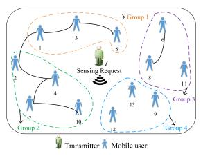
**FIGURE 2.** An example of proposed grouping mechanism with k = 3.
