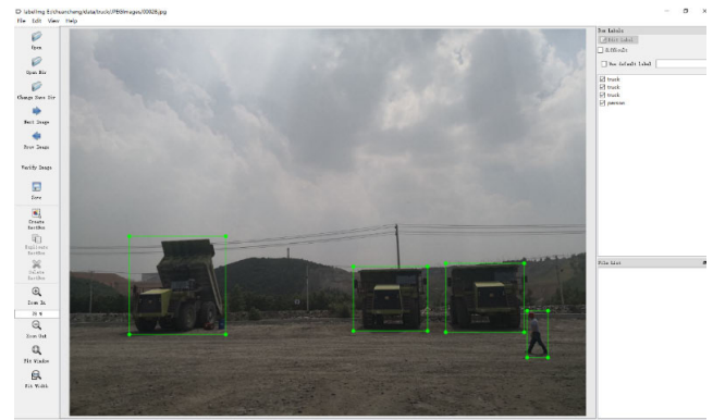
FIGURE 1. Using LabelImg to label the target and then a xml file will be saved which contains position information of the target.
