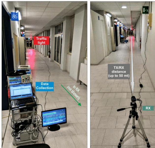
FIGURE 6. Experimental campaign: a standard traffic transmits IOWC signal to a photo-receiver stage equipped with digital active decode and relay block [106].
