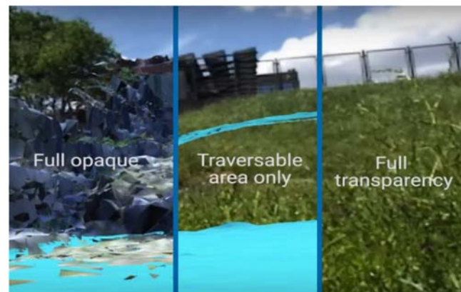
FIGURE 4. Adaptive Transparency VA with 3D reconstruction and traversable area: [left] both opaque, [center] only traversable area opaque, [right] full transparency of live streamed video.
