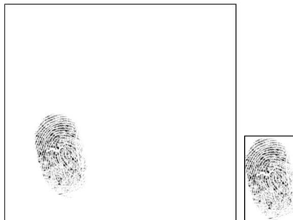
FIGURE 3. The foreground region (181 × 291) extracted from whole fingerprint image (800 × 800) captured from CrossMatch sensor in LivDet2015.
