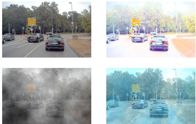
Figure 4: Example of corruptions: original image (top left), brightness, frost and fog corruption (clockwise).
