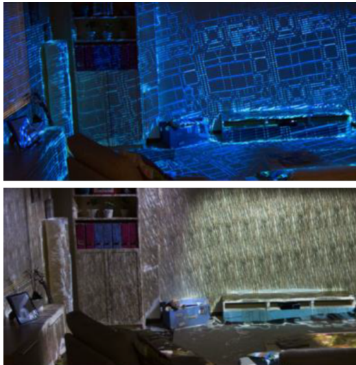
Fig. 6. Using multiple projector-camera systems a whole room is turned into an immersive experience in RoomAlive [166]. Two different visualizations of the same physical room can be seen. Image courtesy of Microsoft Research.
