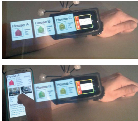
Fig. 17. Top: the field of view of a smartphone is extended by an optical see-through display, in MultiFi [119]. Bottom: A smartwatch is used to select individual icons using touch.
