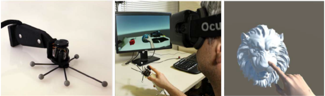
Fig. 8. A haptic controller for VR ( NormalTouch , [22]) is handheld by a user (middle), allowing to render the surface height and normal when touching a virtual object (right). Image courtesy of Microsoft Research.
