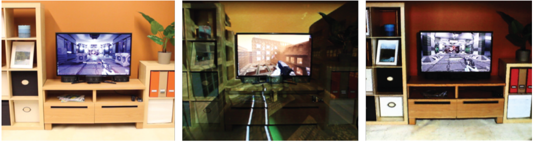
Fig. 5. The area around a TV is augmented using a projector in IllumiRoom [167]. Left: The unmodified scene. Middle: the The field of view of a game is extended beyond the TV boundaries. Right: the appearance of the scene is changed using a cartoon style rendering. Image courtesy of Microsoft Research.
