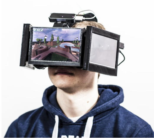
Fig. 15. Multiple Displays around a users head for enhanced interaction in VR [139]. Image courtesy of Jan Gugenheimer.
