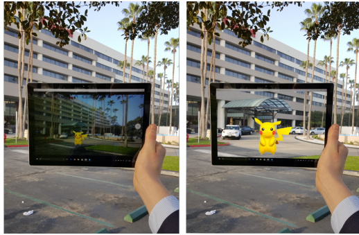
Fig. 4. Effects of device-perspective rendering (left) and user perspective rendering (right) [225].
