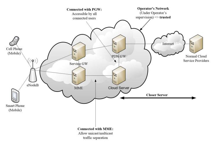
Figure 2.5 Initial phase of OCMCA (without multicast)
