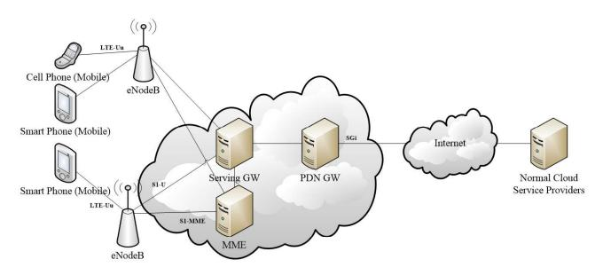
Figure 2.4 EPS network (minimum configuration)
