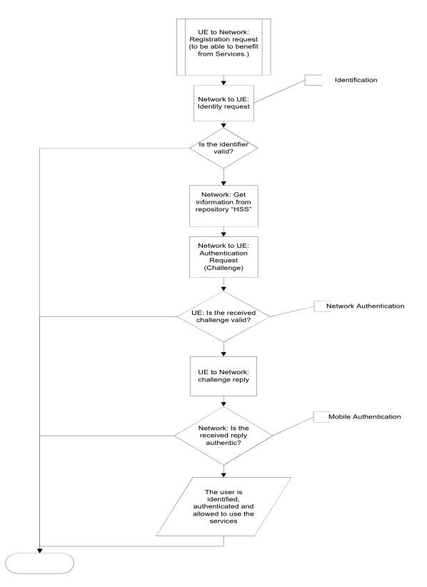
Figure 1.4 Identification and authentication conceptual algorithm
