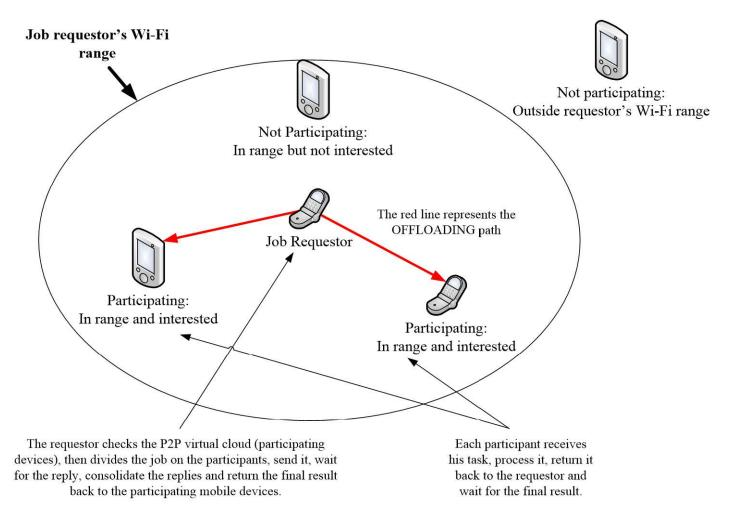
Figure 2.2"Virtual cloud computing provider" architecture
