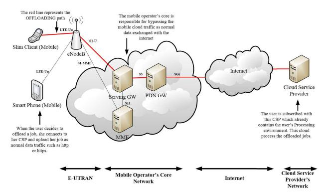
Figure 2.1"Cloud computing with mobile terminals" architecture
