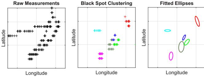
Fig. 7: Steps of the black spot clustering process.
