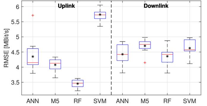
Fig. 6: Resulting data rate prediction performance for different regression models on the *MNO A* data set. ANN: Artificial Neural Network, M5: M5 Regression Tree, RF: Random Forest, SVM: Support Vector Machine
