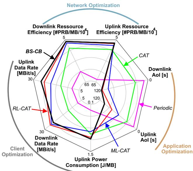
Fig. 19: Summary: Comparison of the average behavior of different performance indicators for the opportunistic data transfer methods in the cellular network of *MNO A*. The axis orientations are chosen such that a large footprint represents a better performance.
