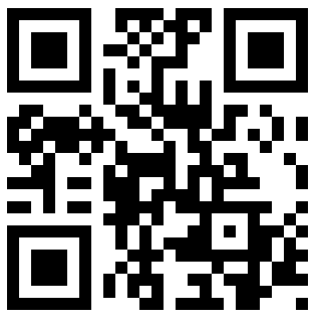
Figure 7—Typical version 2 QR code (this one encodes the text “This is a QR Code”)
