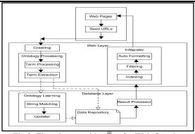
Fig 2: Three layer architecture for Web Crawler
