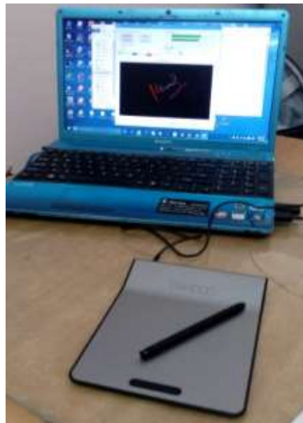
Fig1: System with digital tablet for signature acquisition
