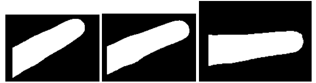
Figure 6. Index ( \alpha ), middle ( \beta ), and ring ( \gamma ) finger masks extracted from a range image.
