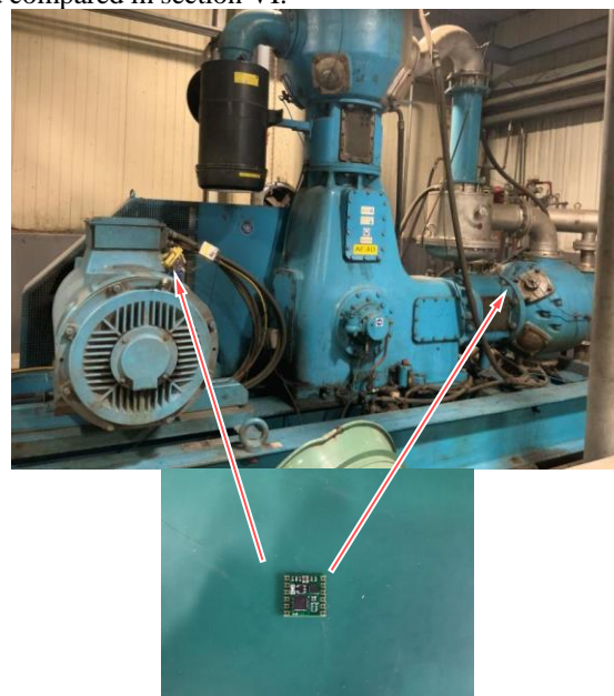
Fig.6 Vibration sensors in different locations in air compressor.
