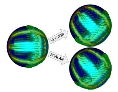
Figure 7.1: Colors represent a scalar field, and the green vectors represent a vector field. Upon rotation, scalar fields transform by simply moving values to another position, while vector fields move and also rotate. Treating vector fields as multi-channel scalars (bottom-right) results in incorrect behavior. The spin-weighted spherical CNNs equivariantly handle vector fields as inputs or outputs.
