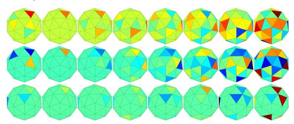
**Figure 4.8:** Localized filters and their receptive fields as we stack more layers. First column shows the filter, second the input, and others are results of stacking group convolutions with the same filter. Top row filter has 12 nonzero elements; middle and bottom have 5. The support for the bottom row contains elements of a 12 element subgroup, so its receptive field cannot cover the full input space.
