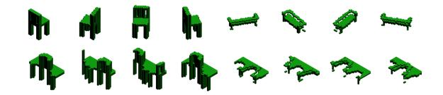
Figure 3.6: Top: rotated voxel occupancy grids. Bottom: corresponding cylindrical representations. Note how rotations around a vertical axis correspond to translations over a horizontal axis.
