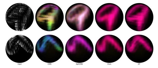
**Figure 7.6:** Input/output samples for the spherical vector field to image task. We show two rotated instances of the same input to highlight that standard CNNs and spherical CNNs do not respect the spherical vector field equivariance, while the SWSCNNs do.
