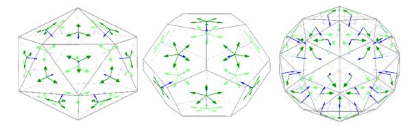
Figure 4.4: Outside-in camera configurations considered. Left to right:  $20 \times 3$ ,  $12 \times 5$ , and  $60 \times 1$ . Blue arrows indicate the optical axis and green, the camera up direction. Object is placed at the intersection of all optical axes. Only the  $60 \times 1$  configuration avoids views related by in-plane rotations.
