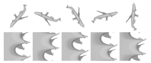
**Figure 4.7:** One subset of in-plane related views from the  $12 \times 5$  configuration and correspondent polar images. Note how the polar images are related by circular vertical shifts so their CNN descriptors are approximately invariant to the in-plane rotation. There are 12 such subsets for the  $12 \times 5$  configuration and 20 for the  $20 \times 3$ ; this allows us to maintain equivariance with 12 or 20 views instead of 60.
