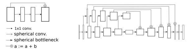
**Figure 5.9:** SCHN architecture. Blocks represent feature maps and arrows, operations. The height of a block represent the spatial resolution and the width, the number of channels. Left: spherical residual bottleneck block. Right: spherical hourglass network.
