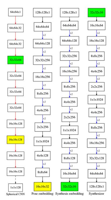
Figure 6.4: Network architectures used in this chapter. Rectangles indicate data dimensions (width x height x channels). *Red arrow:* spherical convolutional residual bottleneck layer; *dashed arrow:* global average pooling; *blue arrow:* residual bottleneck layer; *black arrow:* convolutional layer. Nodes with yellow and green backgrounds are the target embeddings for pose and synthesis, respectively.
