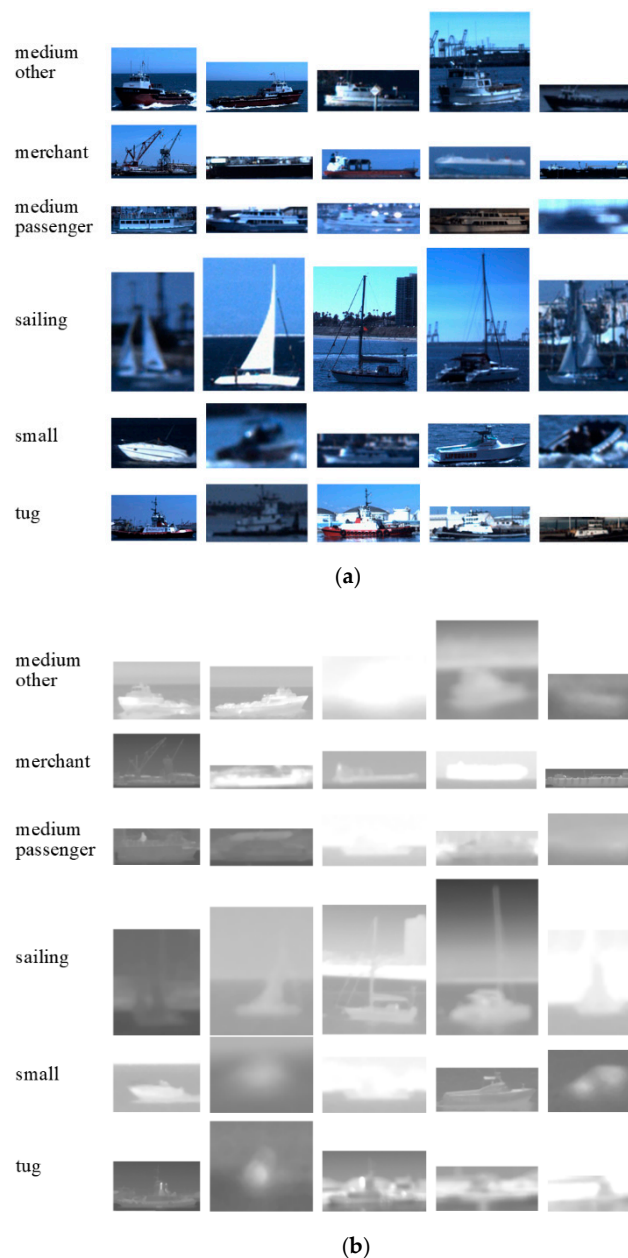
Figure 10. Five visible samples from each of the main classes of the visible and infrared spectra (VAIS) dataset: (a) Visible images; and (b) infrared images.
