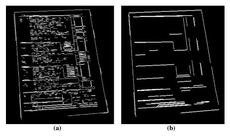
Fig. 5. Length filtering operation. (a): Initial frame. (b): Frame result.
