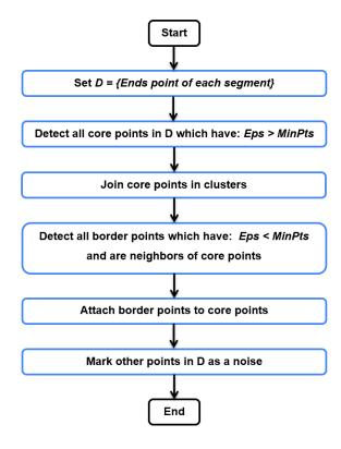
Fig 3. Flowchart of the DBSCAN algorithm.
