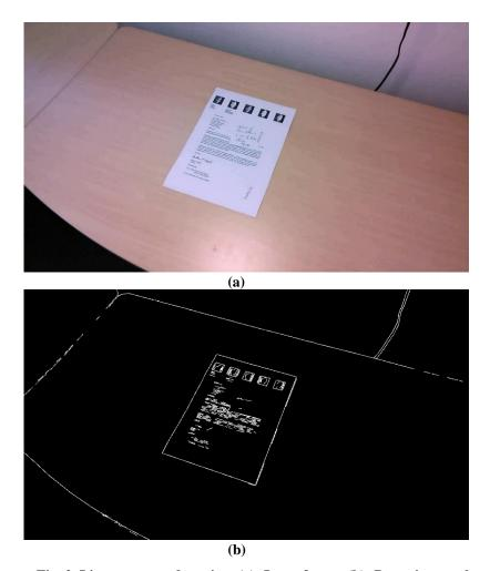
Fig. 2. Line segments detection. (a): Input frame. (b): Detection result.
