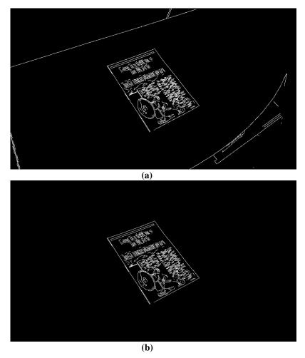
Fig. 4. Application of the DBSCAN clustering algorithm. (a): Initial frames. (b): Result of DBSCAN algorithm.
