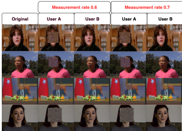
Fig. 4. Sample recovered frames for the semi-authorized (User A) and authorized (User B) (measurement rates 0.6, 0.7).
