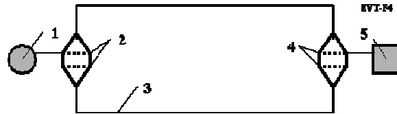
Fig.3. Example of electric line using the AB-Tube s. Notations: 1 – Electric constant-potential generator; 2 – acceleration nets; 3 – electric line from electronic tubes; 4 –brake nets; 5 – customer (user) of electric energy.
