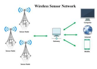
**FIGURE 1.** Data communication in a WSN through gateway.
