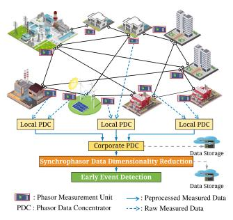
FIGURE 7. Early event detection mechanisms in power grids.
