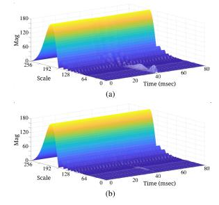
**FIGURE 6.** Simulation results in a IEEE 30-Bus system from [58], where (a) Transmission Line 2-4 is switched-off at t = 30 ms only, (b) Transmission Line 2-5 is switched-off at t = 30 ms only. Both features are extracted at Bus 6.
