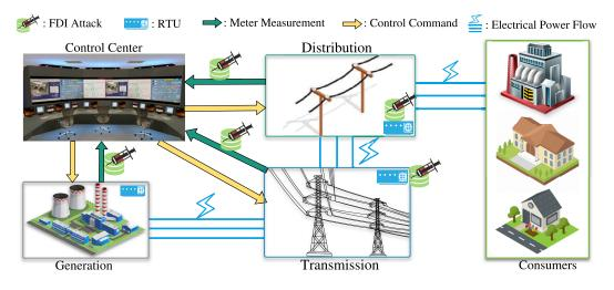
FIGURE 5. FDI attacks on state estimation in a power grids.
