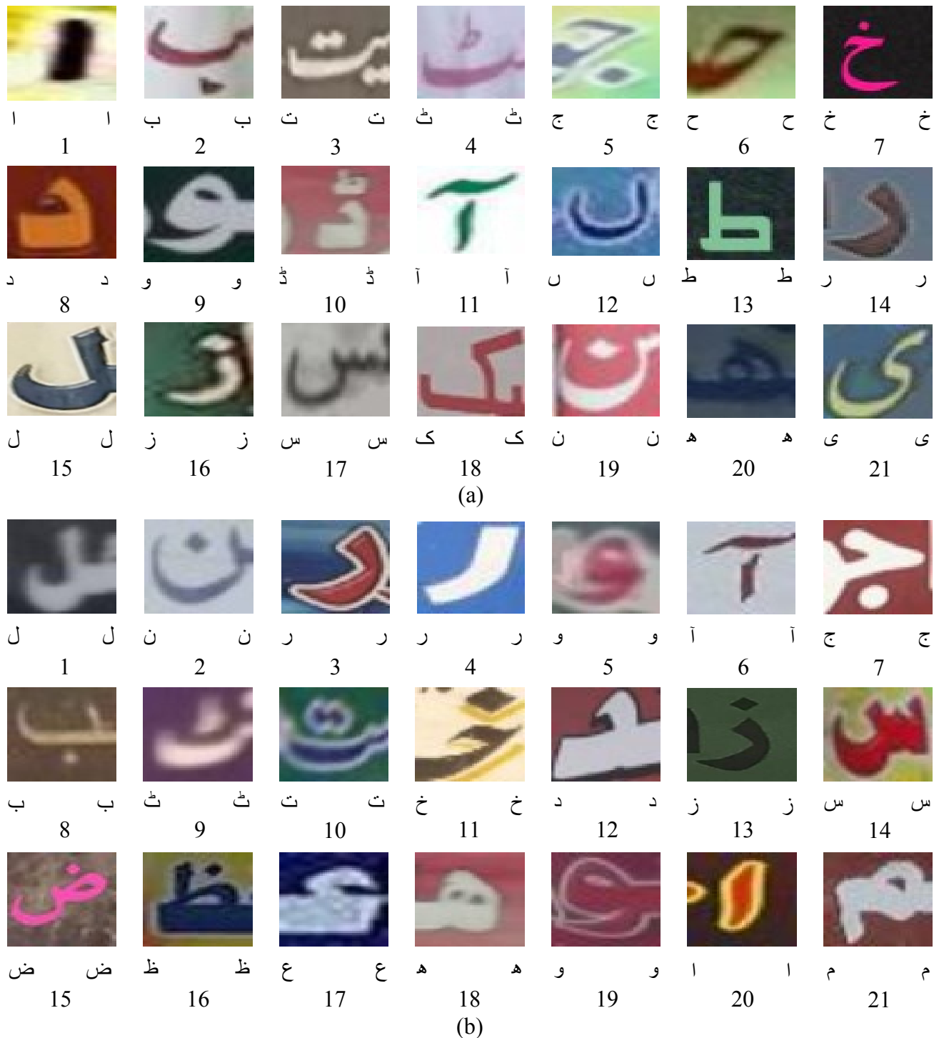
Figure 12: Qualitative results of correctly recognized Urdu characters in natural images: (a) proposed convolutional feature fusion method and (b) HoG method. Labels on the bottom-right are the ground truths, while on the bottom-left are the network predictions.
