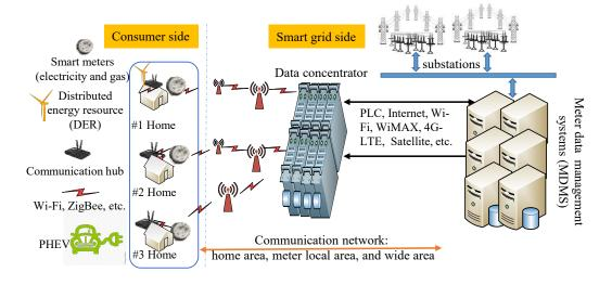
Fig. 3. SG metering network and its components [31].
