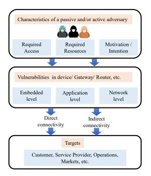
Fig. 6. A high-level threat model in SG metering network.
