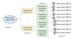
Fig. 11. Hierarchical network of smart grid [115].
