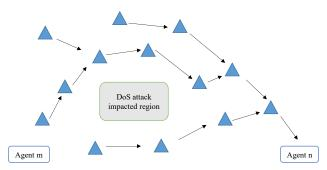
Fig. 9. Data flocking - bypassing DoS region in multiphop routing [143].
