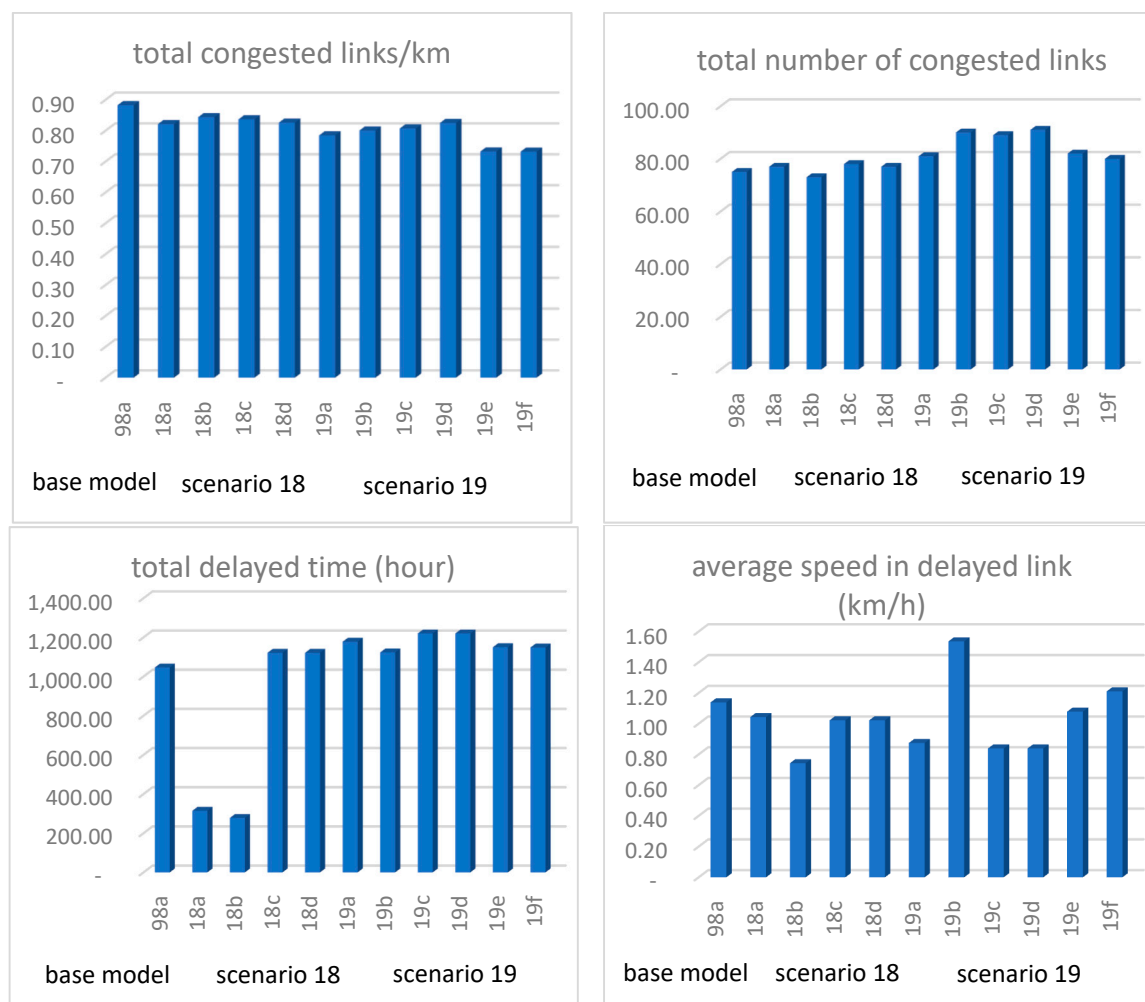
Figure 6. The congested links (only LOS G and H), the speeds and delays per km for all scenarios.
