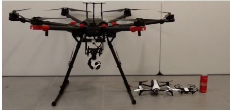
Fig. 1. Mini (DJI Matrice 600 Pro), Micro (Parrot Bebop 2) and Nano (DJI Tello) drones compared to the size of a Coca-Cola can.
