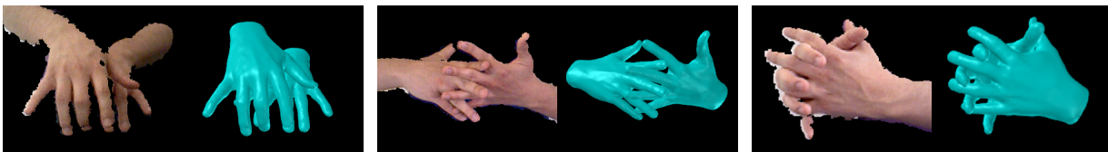
Fig. 1 Qualitative results of our approach for the case of hand-hand interaction. Each pair shows the aligned RGB and depth input images after depth thresholding along with the pose estimate
