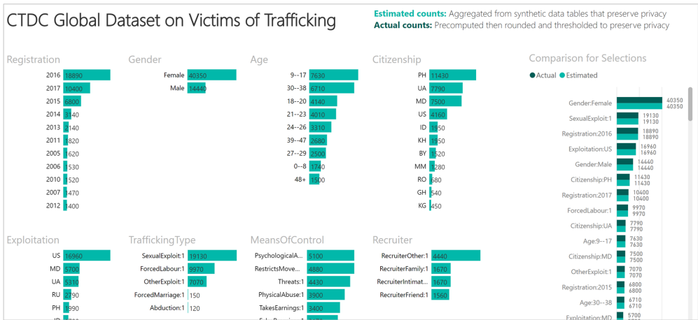
(a) User interface for privacy-preserving analysis of sensitive microdata, generated as a Power BI file. Light bars represent “estimated” counts of attributes in k -synthetic microdata after filtering by user selections. Dark bars represent “actual” reportable counts precomputed from sensitive data and retrieved for comparison. The synthesis algorithm ensures that “estimated” counts are initially equal to “actual” counts, which preserve privacy through the use of a minimum reporting threshold k and fixed rounding precision p .
