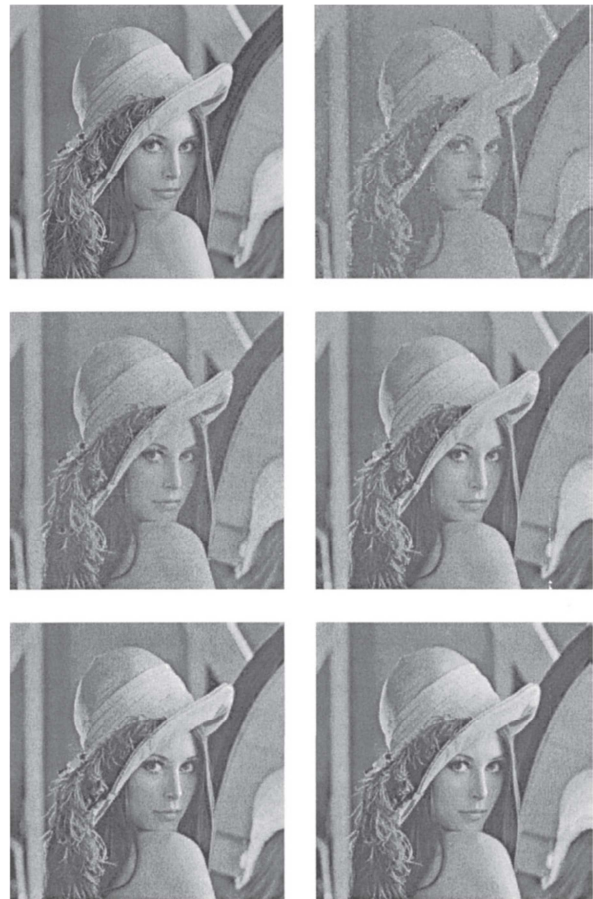
Figure 5. Original Lena and images obtained using FBPNN with PSNR=21.16, 26.42, 30.35, 32.22, 32.79 [dB], respectively [2]. © Springer - Verlag.
