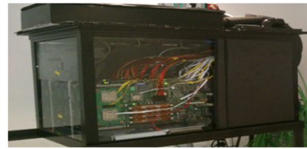
Fig. 20. Immersion cooling container prototype in Orange Labs
