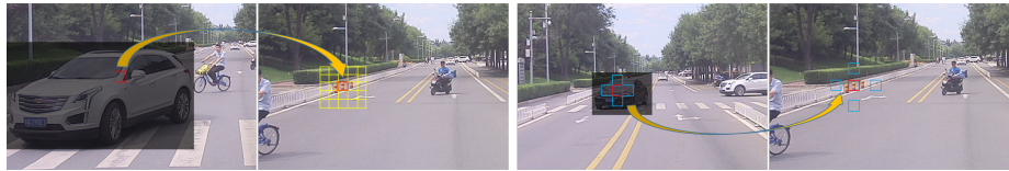
Fig. 5. Left image pair: potential color choices for a target pixel. a pixel within inpainting region find its candidate pixel (red box) from a source image. A small window of pixels around this candidate (yellow boxes) are all potential colors to fill the target pixel. Right image pair: the 4 neighbors of a target pixel are not necessarily neighbors in the source image due to perspective change. In order to get neighbor colors, we need to warp neighbor pixels into the source image by their depth value.
