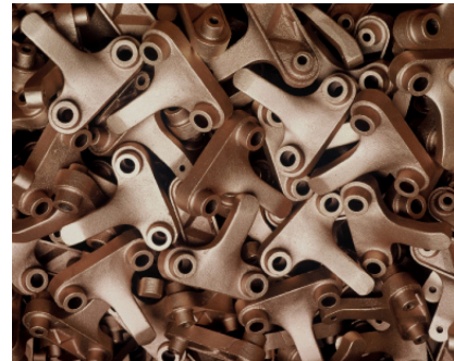
Fig. 2. Objects supplied in bulk are stacked randomly in a bin. An object detection and pose estimation algorithm is needed to determine the six degree of freedom pose of a pickable object, so that it can be grasped by the robot.
