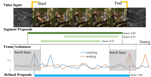
Figure 1: Our proposed MGG can generate segment proposals and frame actionness simultaneously, which helps discover information about possible actions at both the coarse and fine levels. By temporally adjusting the boundaries of the segment within the search space determined by the computed frame actionness, MGG can yield refined action proposals with both high recall and precision.
