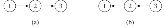
Fig. 3: Constructing the transpose graph: (a) directed plant graph \mathcal{G}_p(\mathcal{V}, \mathcal{E}_p) , (b) the transpose graph of \mathcal{G}_p .
