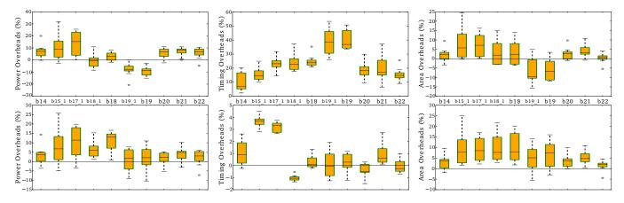
Fig. 19. Distribution of layout cost for all 18 different structures we explored on various benchmarks. Top: without any optimization; bottom: with buffer insertion applied (only outside of the structures). Note that the same benchmarks are applied for the top and bottom plots; benchmark labels are accordingly placed between those plots. Also note the different scales for each plot. Each boxplot represents ten runs.
