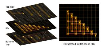
Fig. 9. Obfuscated switchbox, embedded in two RDL layers, exemplarily for bottom-to-top drivers. Each driver pin (downwards triangle) can connect to any sink pin (upwards triangle). All F2F ports are aligned with the pins of the switchbox here, for simplicity, whereas the top-tier ports are randomized in reality.
