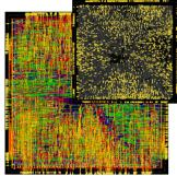
Fig. 10. Layout snapshots of bottom/top tier (left/right) for *b22*. The insets show the corresponding F2F vias.
