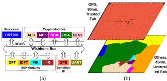
Fig. 6. (a) Architecture of the DARPA Common Evaluation Platform [36]. The GPS block is considered the sensitive IP; it is thus to be delegated to the trusted fabrication. (b) Heterogeneous 3D implementation, with colors corresponding to modules in (a).
