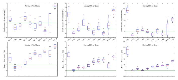
Fig. 11. Impact of randomly assigning gates on performance (top) and power (bottom). Each boxplot represents ten runs. Note that the same benchmarks are applied for the top and bottom plots; benchmark labels are accordingly placed between those plots.
