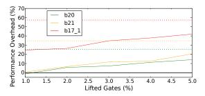
Fig. S1. Performance degradation when lifting gates in 3D from the 45nm tier to the 180nm tier. Dotted lines indicate the critical-path delays for the 180nm 2D baseline setup. See also Table S1 and its footnote.
