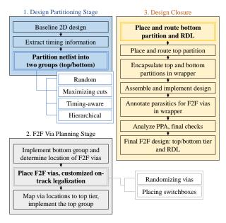
Fig. 7. Our CAD flow for F2F 3D ICs, implemented in *Cadence Innovus*. Security-driven steps for IP protection are emphasized in bold.
