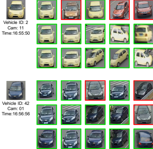
Figure 8: Example vehicle re-identification results (top5) by our proposed approach. The true positive is in green box otherwise red. The three rows are results of Siamese-Visual, Siamese-CNN and Siamese-CNN+Path-LSTM.
