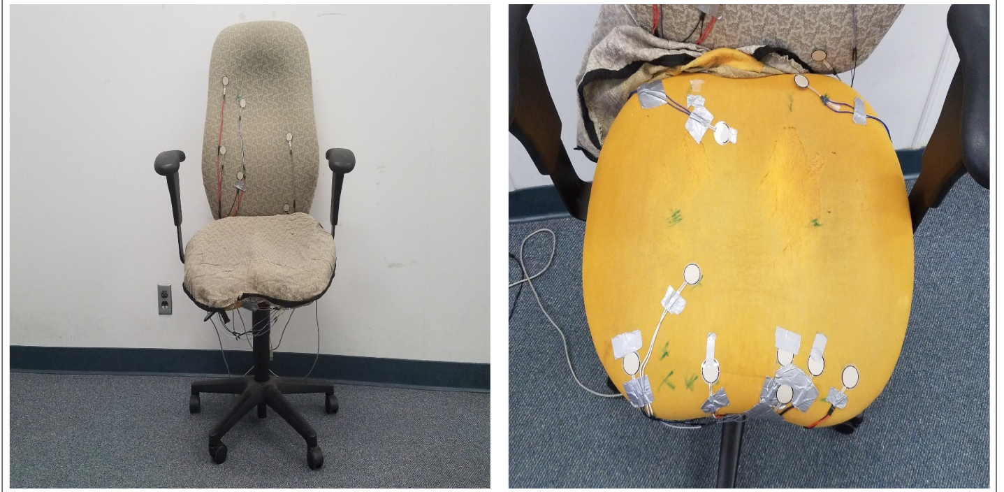
Fig. 1: The PoPa prototype chair: (a) as seen by user, and (b) uncovered seat-bottom sensor placements.
