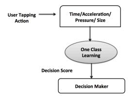
Figure 5: Non-Intrusive User Verification Architecture
