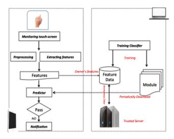
Figure 9: Architecture of Re-authentication Model
